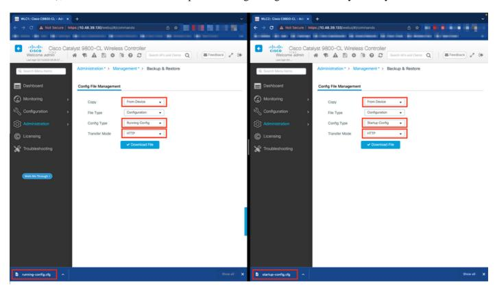
In this example, both startup (left-hand side) and configuration (right-hand side) are directly downloaded, through HTTP, on the device that hosts the browser used to access the GUI of the WLC. One can easily tweak the transfer mode and destination of the file to be backed up, with the Transfer Mode field.
