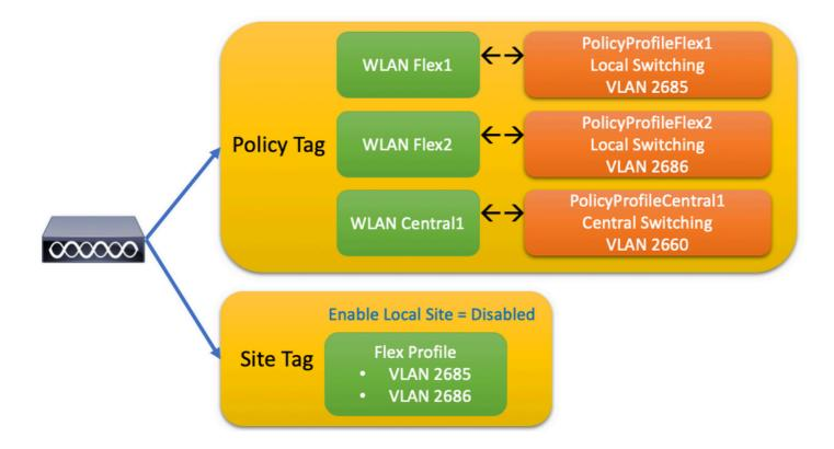
To configure a FlexConnect Local Switching Service Set Identifier (SSID), here are the general steps to follow:
