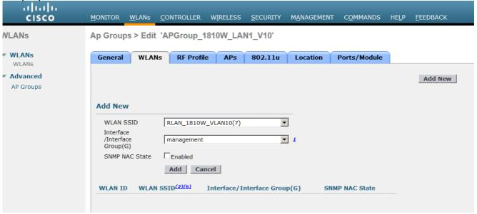
**Note**: AP level configuration of the RLAN-Port mapping is not currently supported. However, the GUI does have a section to enable/disable the ports at AP level. Any changes there will override the Group level, and *should be left at defaults*.
