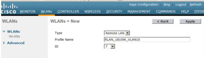
**Note**: MAC filtering is enabled by default when a new RLAN is created. Be sure to disable if not used.
