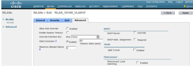
3. Check the **FlexConnect Local Switching** checkbox. In the VLAN Id field enter the VLAN ID to which this RLAN will map LAN Port data locally at the AP. Click **Apply** in order to save changes.
