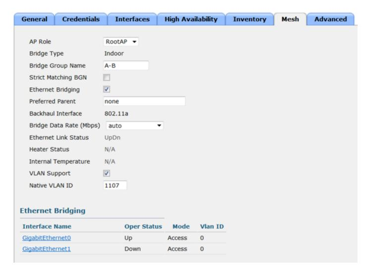
First Mesh AP of the daisy chain. This is considered the Primary of the chain. It uses its 5Ghz radio to connect to the wired Rap. Note that daisy chaining is enabled on this AP.
