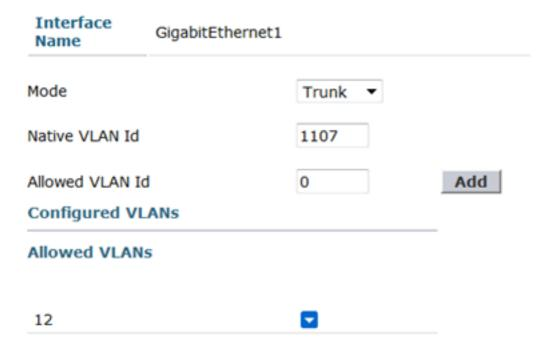
Core switch port configuration for the Root AP
