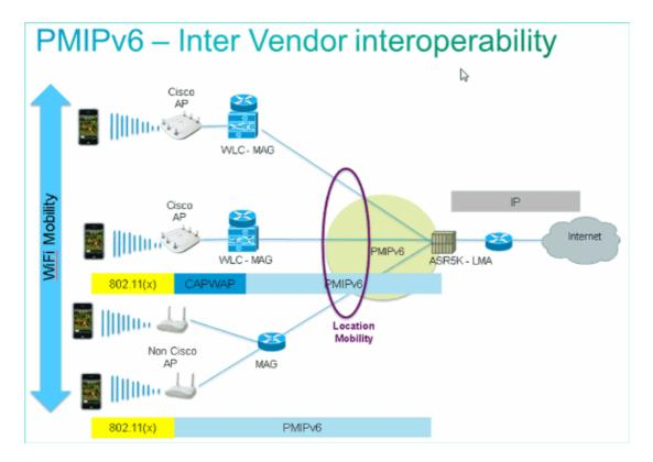
PMIPv6 facilitates IP mobility by keeping these mobility parameters constant throughout the PMIPv6 domain:
