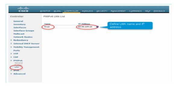
Once the above is done, the static PMIPv6 GRE tunnel between the WLC-MAG and LMA will be up.
