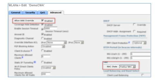
*Note*: RADIUS Network Admission Control (NAC) is not supported when the FlexConnect AP is in disconnected mode. Thus, if the FlexConnect AP is in standalone mode and loses connection to the WLC, all clients are disconnected, and the SSID is no longer advertised.
