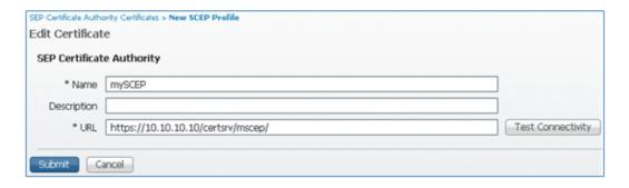
101. Click *Test Connectivity* in order to test connectivity of the SCEP connection.
