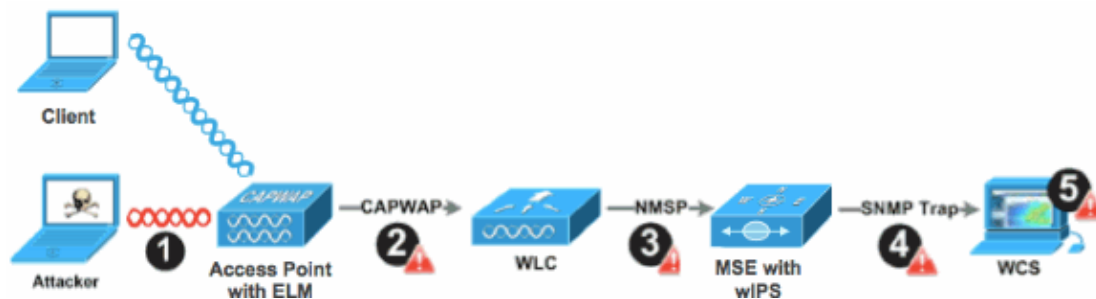
Figure 3 – Threat Detection and Alarm Flow
