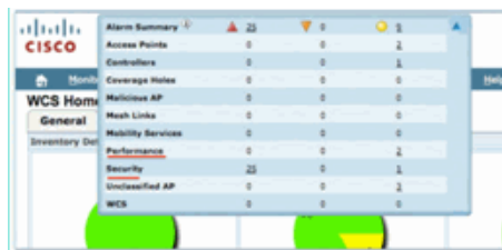
Figure 29: Alarm Summary panel
