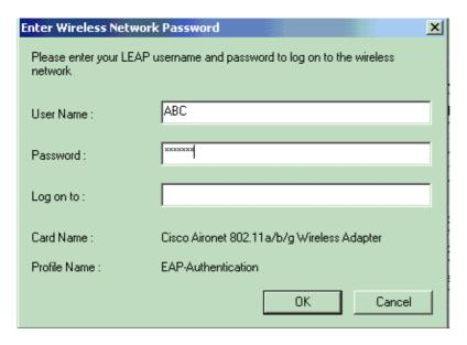
The Lightweight AP and then the WLC pass on the user credentials to the external RADIUS server (Cisco Secure ACS) in order to validate the credentials. The RADIUS server compares the data with the user database and provides access to the wireless client whenever the user credentials are valid in order to verify the user credentials. The Passed Authentication report on the ACS server shows that the client has passed the RADIUS authentication. Here is an example:
