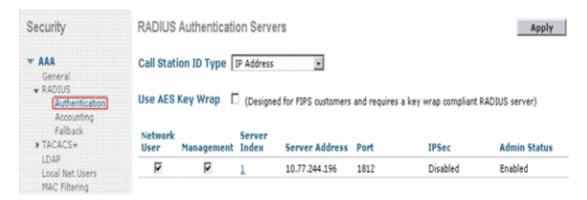
RFC 3576 is supported on the Cisco CNS Access Registrar (CAR) RADIUS server, but not on Cisco Secure ACS Server version 4.0 and earlier.
