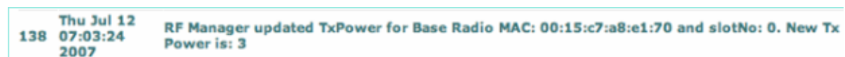
Figure 18: The Tx Power trap log indicates the new power-level of operation for the specified radio.
