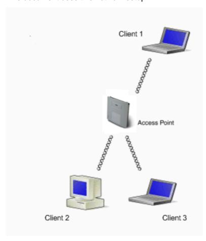
The network diagram is three Aironet 802.11a/b/g Client Adapters that are connected to a 1200 AP. This document depicts the configuration of the client adapters to communicate with each other via wireless interface through the AP.
