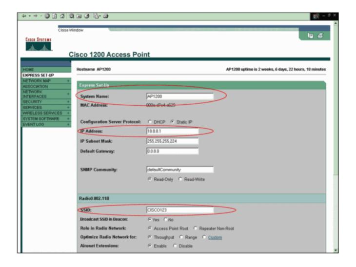
Enter the configuration parameters in the appropriate fields in the Express Setup window.
