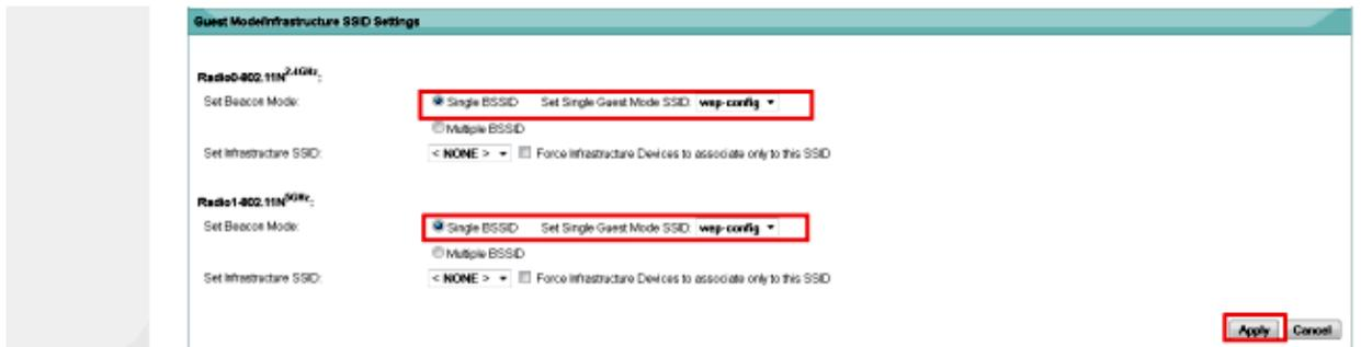
7. Navigate to the network, and enable the radios for **2.4 GHz** and **5 GHz** in order to get them running.
