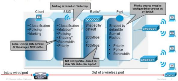
This configuration example focuses on the wireless aspect of QoS configuration and marks traffic at wireless client level. Once the marking portion has been completed, you need to allocate bandwidth; here, 6 Mbps of bandwidth is allocated to voice traffic flows. (While this is the overall bandwidth allocation for voice, each call would consume less – for example, 128 kbps.) This bandwidth is allocated with the *police* command in order to reserve the bandwidth and to drop traffic in excess.
