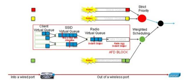
This configuration example places voice into the first priority queue and video in the second priority queue through use of the *priority level* command. The rest of the traffic is allocated the rest of the port bandwidth.
