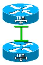
We have configured one NAS to source the clock (free-running). The other is configured to derive clock from the line.
