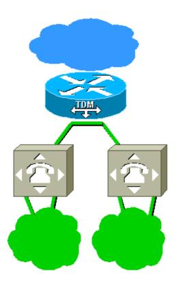
The NAS is connected to two TDM switches, which are in different TDM networks. The networks are not directly clocked in common. However, they are plesiochronous, and both use such accurate clocks that they are, for all practical purposes, synchronized. As with Example 2, configure the NAS to derive clocking from one of the lines, and to fail over to the other line.
