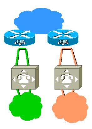
Here, we have two unsynchronized TDM networks separated by a packet network path. This prevents the occurrence of slips on the TDM spans. However, if we build a circuit between the two networks with a Voice over IP (VoIP) link through the packet network, synchronization problems can occur.
