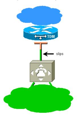
The NAS is connected to a single TDM switch, but is not synchronized to that switch. The NAS can use the local oscillator (free running) or be synchronized to some other source. There will be slips on the interface between the NAS and the TDM switch. The solution is to configure the NAS to derive the clock from the line.
