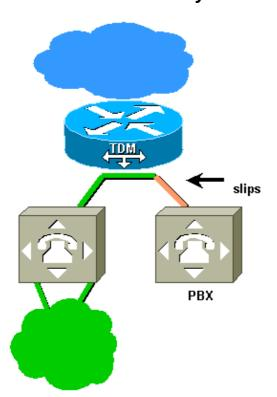
The NAS is configured to derive clocking from the switch on the left. The private branch exchange (PBX) uses a different source for synchronization, and the orange span on the right will therefore experience slips. The solution is to reconfigure the PBX to derive clocking from the line to the NAS.
