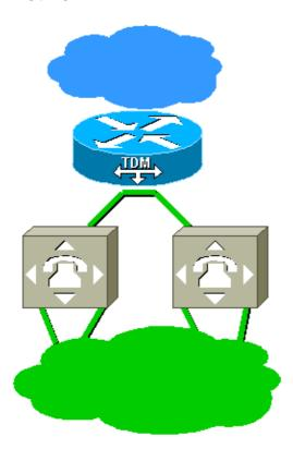
The NAS is connected to two TDM switches. The two switches are in the same TDM network, and are synchronized to each other. Configure the NAS to derive clocking from one of the lines, and to fail over to the other line.
