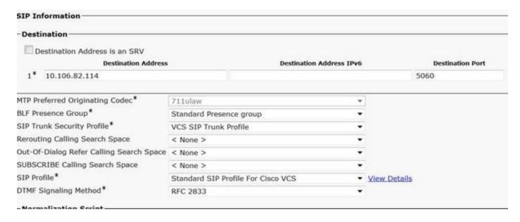
**Note**: A new Trunk Security profile is created which listens on 5065 port. It is assigned to this new SIP trunk pointing to Expressway-C because Expressway-C is already configured to send Jabber Un-secure registrations on 5060 to CUCM when Jabber user logs in via MRA. If you use the default Trunk Security profile, then jabber logged in via MRA fails to register on port 5060 of CUCM.
