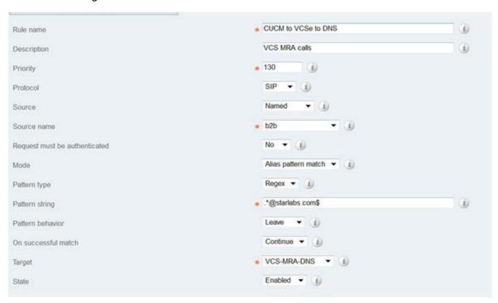
Step 10. Once the Call hits the DNS Zone, Expressway-C does a DNS SRV Lookup for \_sips.tcp.starlabs.com, \_sip.\_tcp.starlabs.com and \_sip.\_udp.starlabs.com against the Public DNS Server.
