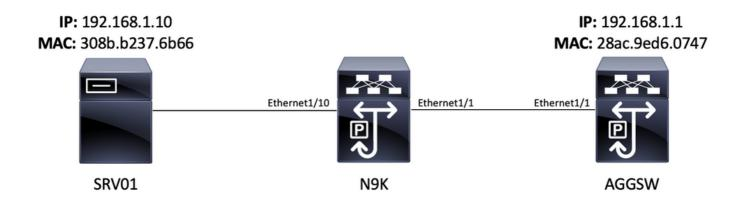
An Internet Control Message Protocol (ICMP) packet sourced from server SRV01 in VLAN 10 (192.168.10.10) is destined for the VLAN 10 gateway 192.168.10.1. A SPAN-to-CPU monitor session will be used to confirm that this ICMP packet traverses device N9K (a Cisco Nexus 93180YC-EX that runs NX-OS software release 9.3(3)), which acts as a Layer 2 switch that connects SRV01 to AGGSW in VLAN 10.
