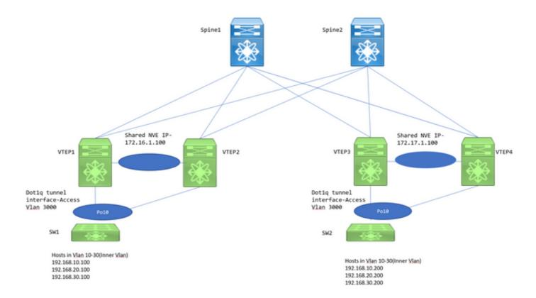
VTEP1, VTEP2, VTEP3, and VTEP4 are two vPC VTEP pairs configured in such a way that the inner dot1q tags from downstream switches are preserved and when VXLAN encapsulated, use outer VLAN ID's VXLAN VNID in order to send over to the remote VTEP. All VTEPs are N9K-C93180YC-EX.
