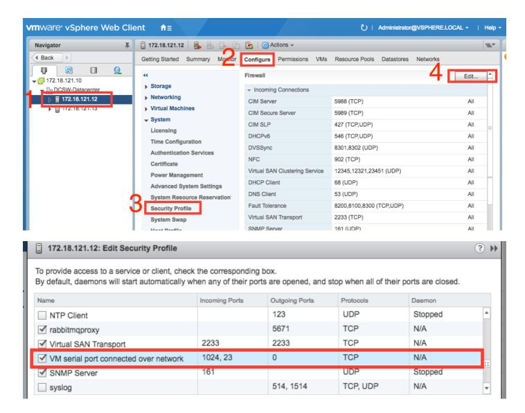
2. Under the VM **Edit Settings** menu add a network backed serial port to the NX-OSv 9000 Virtual Machine. The NX-OSv 9000 VM must be turned off to add this.
