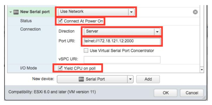
**Note**: the interface IP address specified for the port URI must be the VMkernel interface IP address that is used for managment services on the ESXi host the VM currently resides on. The port number may be any TCP port above 1024 that is not currently in use. Be sure to pick a port that is not used for any other VMkernel service such as vMotion, etc.
