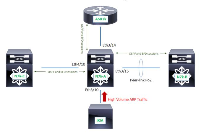
The following output shows an increase of input traffic on interface Ethernet 3/10, where the IXIA Traffic Generator is connected. These are broadcast ARP packets received in vlan 6
