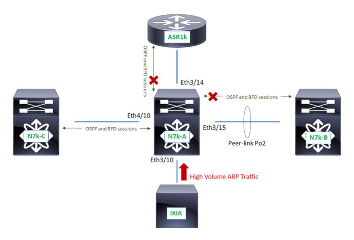
The following outputs confirm the impact of an ARP packet storm on both BFD and OSPF sessions on the module in slot 3. Contrary to this BFD and OSPF session(s) on the module in slot 4 are established and remain stable.
