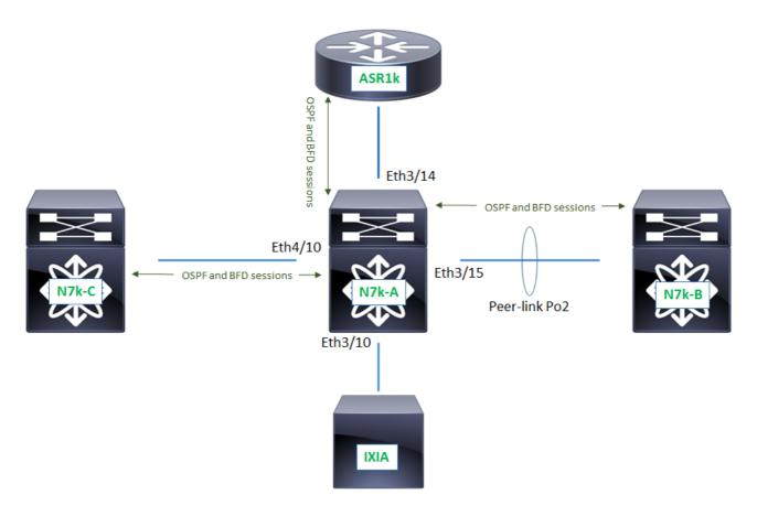
Here N7k-A is used as Device Under Test (DUT). DUT is a Nexus 7009 switch with the following hardware configuration
