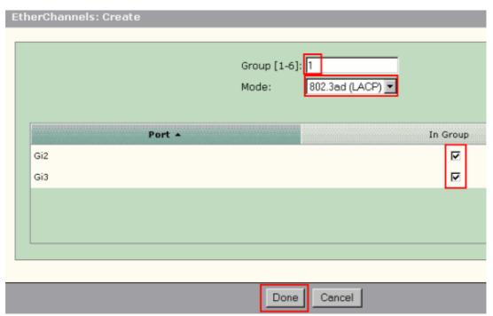
7. If you have chosen LACP protocol to negotiate the channel, then configure the remote switch as this output shows:
