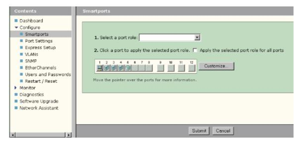
From the Smartports window, you can see which Smartports role is applied to each port. Move the pointer over a port to display its port number, Smartports role, and VLAN ID (VLAN membership).
