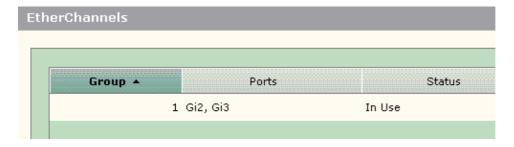
Issue the **show etherchannel summary** command in the Cisco 3750 switch to verify the status of the EtherChannel configuration. The Protocol field in the output displays LACP if it is used to negotiate the channel, blank or otherwise.
