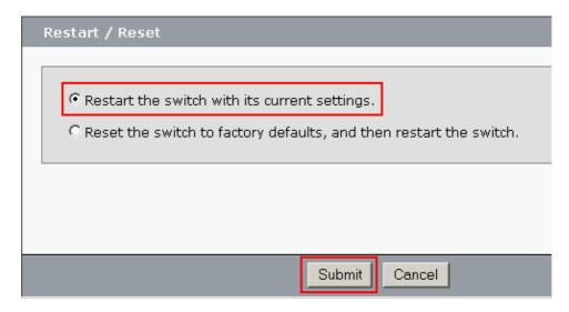
The switch automatically reloads in 60 seconds. A counter displays the time that remains for the reload.
