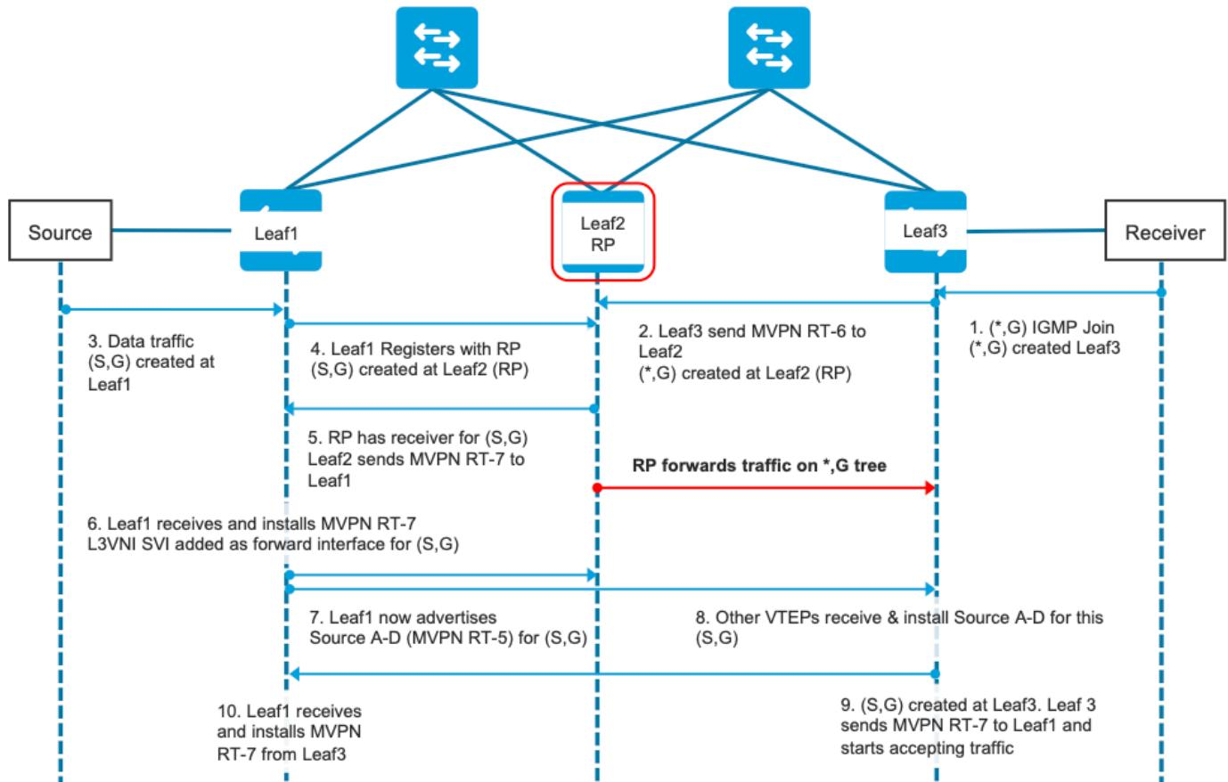
**Step EVPN (Leaf-03):** EVPN Type-5 from RP is learned on LHR. This is required for the receiver VTEP to create an MVPN Type-6 route
