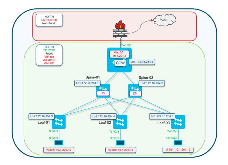
Protected configuration keyword is applied on the Leaf switches. The CGW is a promiscuous device and installs all mac addresses.
