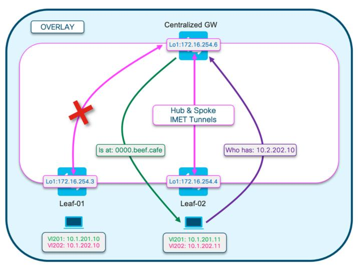
This diagram is to help visualize the flow of the ARP resolution process described in this section.
