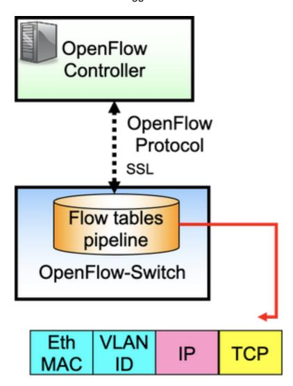
OpenFlow is the protocol between the controller (control plane) and the ethernet switch (data plane). The switch has flow tables arranged into a pipeline and the flows are rules to examine the packets.
