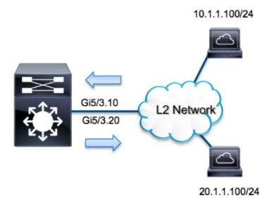
In this example, the 6500 acts as a *router on a stick* in order to route traffic between hosts on VLAN 10 and VLAN 20. ELAM is used in order to validate that an Internet Control Message Protocol (ICMP) request from host *10.1.1.100* received on port *G5/3* of VLAN 10 is successfully routed back to *20.1.1.100* on port *G5/3* of VLAN 20.
