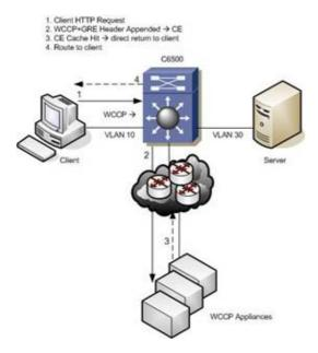
WCCP L3 operation involves the use of GRE as an encapsulation method. Redirected packets are
