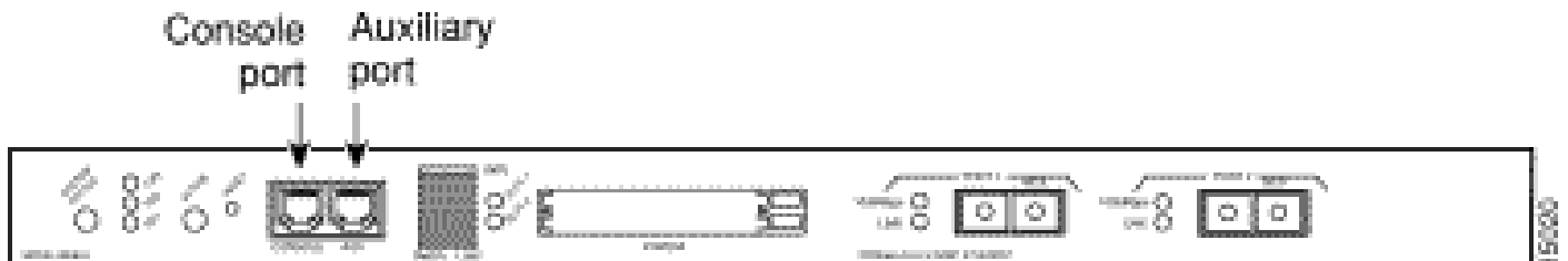
Figure: Console and AUX Port Connectors
