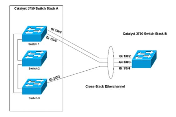
In this network diagram, there are two Catalyst 3750 Switch stacks, Stack A and Stack B. Stack A has three switch members, and Stack B has only one switch member. The EtherChannel is formed with two ports on Switch 1 and one port on Switch 3 of Stack A. These ports connect to the three ports in Stack B.
