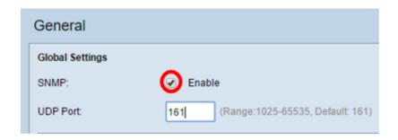
Step 3. Enter the UDP port number in the *UDP Port* field. The SNMP agent checks this port for access requests. The default port is 161.
