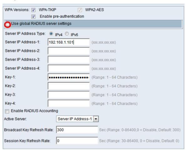
Step 6. (Optional) Click the radio button for the correct **Server IP Address Type**.
