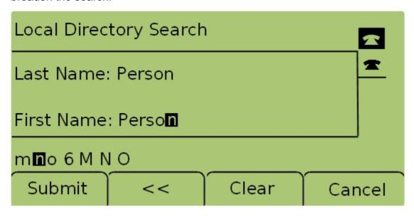
Step 5. Navigate to the First Name field with the navigation keys. Enter the first name of a person to search for in the First Name field by pressing the corresponding key for that letter. Repeatedly press that same key to select the desired letter.
