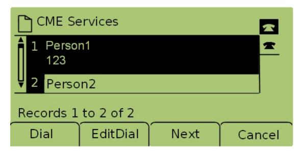
Step 7. The name and extension number of each match found is shown. Use the navigation keys to scroll up and down to view each entry.
