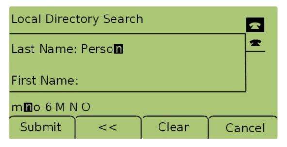
Step 4. Enter the last name of a person to search for in the Last Name field by pressing the corresponding key for that letter. Repeatedly press that same key to select the desired letter.
