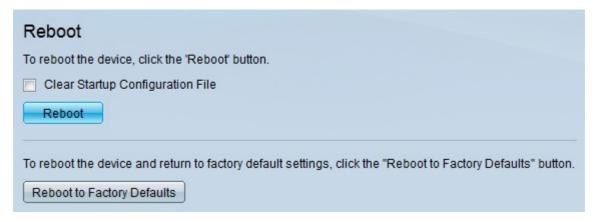
Step 2. (Optional) Check the **Clear Startup Configuration File** check box to delete the startup configuration once the switch is rebooted. With this option chosen, the switch essentially performs a factory default reset since both the running and startup configurations will be deleted on reboot.
