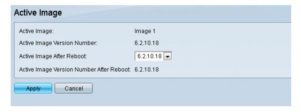
Step 2. Select the desired firmware version from the *Active Image After Reboot* drop-down list.
