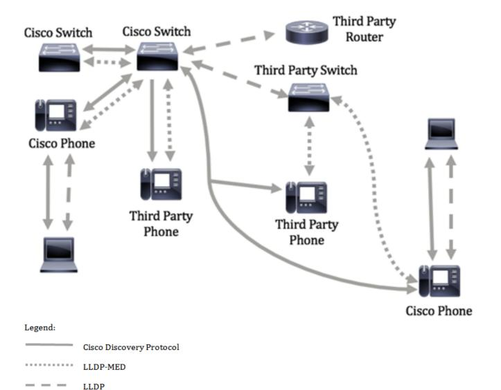
The diagram below shows a scenario wherein control in protocols have already been configured accordingly: CDP is used between Cisco devices while LLDP-MED is used between Cisco and third party devices.
