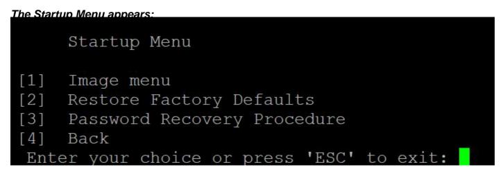
Step 3. Press 3 to select option [3] Password Recovery Procedure. This will reset the password to null.
