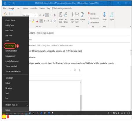
In the Device Manager, you would look to see what COM port is given to the USB adapter. In this case you would need to use COM4 for the Serial line to make the connection.
