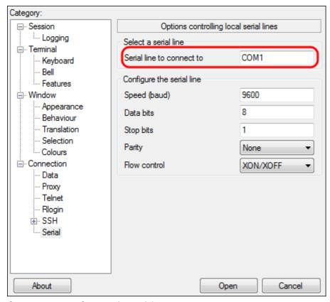
Step 6. In the *Speed (baud)* field, enter the digital transmission speed that is compatible with the switch. For 300 and 500 Series Managed Switches, the speed must be set to **115200**.
