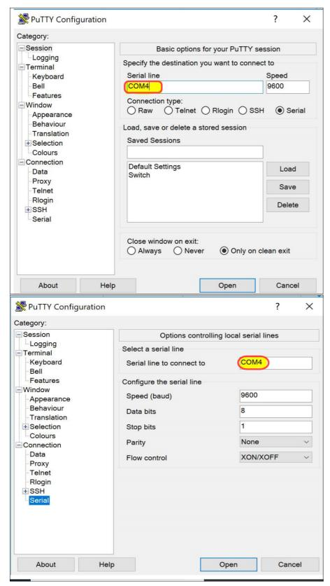
Step 2. Open the PuTTY application. The PuTTY Configuration window opens:
