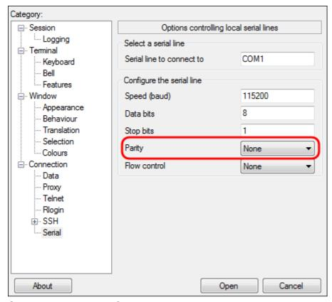
Step 10. In the *Flow Control* drop-down menu, select the method of preventing data overflow. The recommended method for preventing data overflow is **None**.
