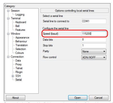
Step 7. In the *Data bits* field, enter the number of data bits used for each character. The recommended value is **8**.
