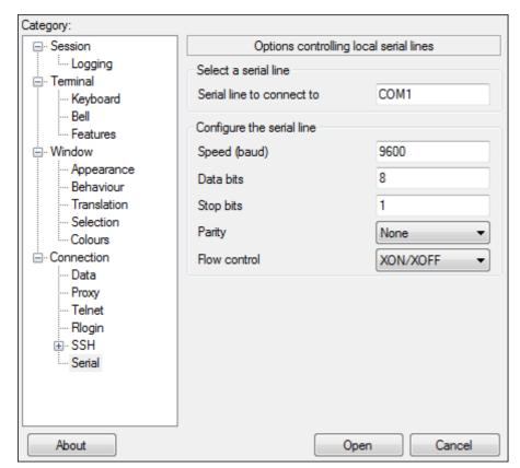
Step 5. In the *Serial line to connect to* field, enter the COM port that your device is connected to. The default COM port is COM1.
