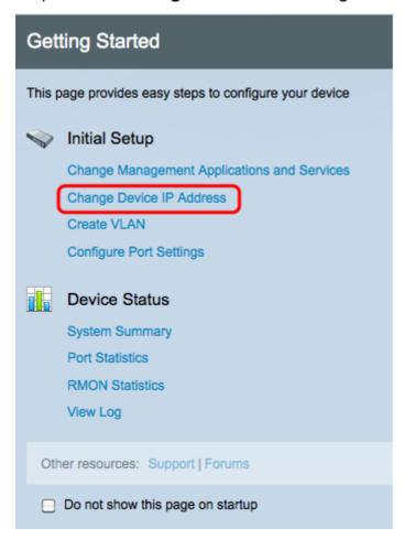
Step 3. Click Change Device IP Address to change the IP address of the switch. The IPv4
