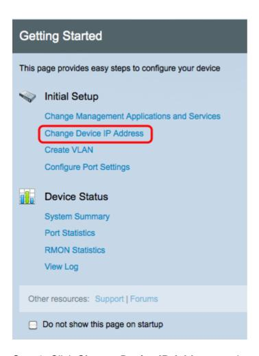
Step 3. Click **Change Device IP Address** to change the IP address of the switch. The *IPv4 Interface* page opens:
