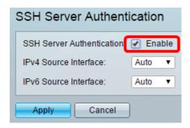
Step 3. (Optional) In the IPv4 Source Interface drop-down list, choose the source interface whose IPv4 address will be used as the source IPv4 address for messages used in communication with IPv4 SSH servers.
