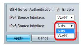
**Note:** In this example, the Auto option is chosen. The system will take the source IP address from the IP address defined on the outgoing interface.
