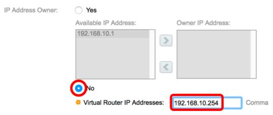
**Note:** In this example, No is chosen and the IP address entered is 192.168.10.254. This indicates the IP address on the virtual router.
