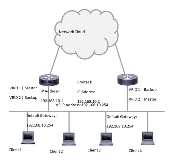
For virtual router 2, Router B is the owner of IP address 192.168.10.2 and virtual active router, and Router A is the virtual router standby to Router B. Clients 3 and 4 are configured with the default gateway IP address of 192.168.10.254.
