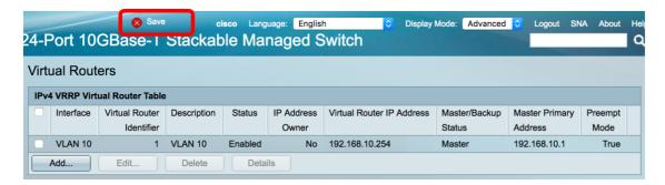
**Note:** The active/standby Status area of the IPv4 VRRP Virtual Router Table should display the status of the virtual router that you have configured. If you intend to configure a standby virtual router, the status should display as standby.
