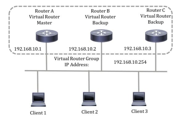
Because the virtual IP address uses the IP address of the physical Ethernet interface of Router A, Router A is the active router (also known as the IP address owner). As the active router, Router A owns the virtual IP address of the VRRP group and forwards packets sent to this IP address. Clients 1 through 3 are configured with the default gateway IP address of 192.168.10.254.
