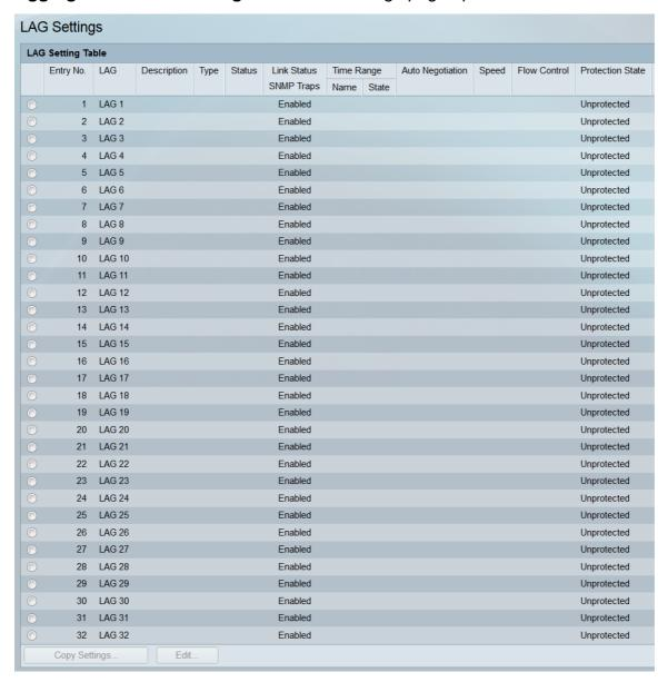
Step 2. The *LAG Setting Table* displays information on all LAGs currently configured on the switch. Select a LAG's radio button and click **Edit...** to edit its settings in the *Edit LAG Settings* page.
