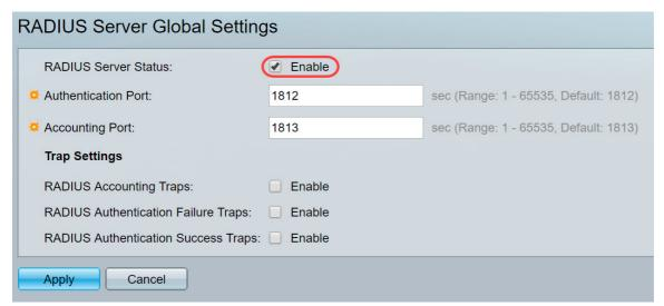
Step 3. To generate traps for RADIUS accounting events, logins that failed, or for logins that succeeded, check the desired **Enable** checkbox to generate traps. Traps are system events messages generated via Simple Network Management Protocol (SNMP). A trap is sent to the SNMP manager of the switch when a violation occurs. The following trap settings are:
