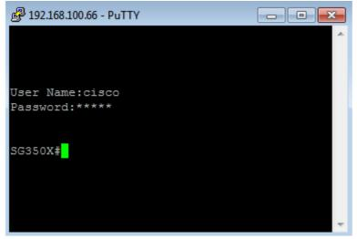
You have now successfully accessed the CLI or the web-based utility of the switch using IPv4 management interface IP address.
