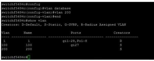
**Note:** VLAN 1 is the default VLAN, which by default, includes all possible ports on the switch. Ports that are numbered with *gi* are Gigabit Ethernet (individual links). Ports that are numbered with *fa* are Fast Ethernet (individual links). Ports that are numbered with *Po* are port-channels (a group of Ethernet links).
