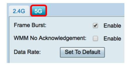
Step 2. Check the **Enable** Frame Burst check box to enable the radio to rapidly send a series of frames in succession for a brief period of time. Frame burst enhances the ability of a client to upload data at higher throughputs with the use of inter-frame wait intervals to burst a sequence of up to three packets before it has to wait for a required period. The default is unchecked.
