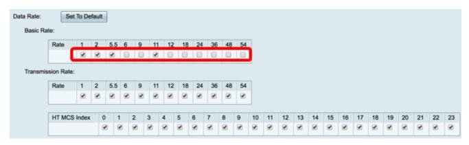
Step 7. In the Transmission Rate area, check the check boxes of the necessary rates at the bandwidth of your wireless network. The default setting is all check boxes are checked.
