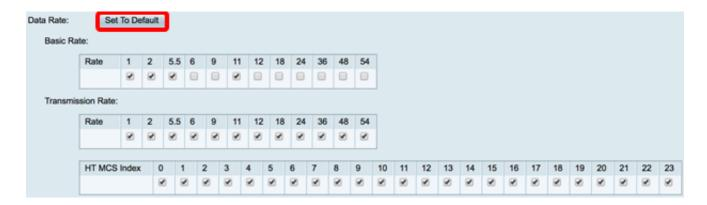
Step 6. In the Basic Rate table, check the check boxes of applicable rates in Megabits per second (Mbps) at which the 2.4 GHz radio will broadcast. The default rates are 1 Mbps, 2 Mbps, 5.5 Mbps, and 11 Mbps.
