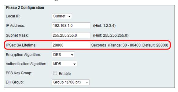
Step 14. From the *Encryption Algorithm* drop-down list, choose the appropriate encryption method to encrypt the Pre-Shared key in Phase 2. AES-128 is recommended for its high security and fast performance. The VPN tunnel needs to use the same encryption method for both of its ends.
