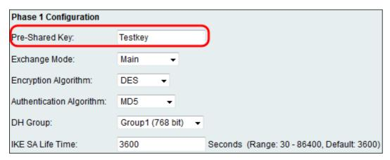
Step 5. From the *Exchange Mode* drop down list, choose the mode for the IPSec VPN connection. **Main** is the default mode. However, if your network speed is low, choose the **Aggressive** mode.
