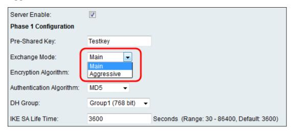
**Note:** Aggressive mode exchanges the IDs of the end points of the tunnel in clear text during the connection, which requires less time to exchange but is less secure.
