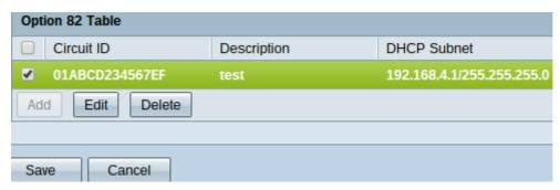
Step 1. To modify a circuit ID name and description check the check box next to it. The entry is highlighted.
