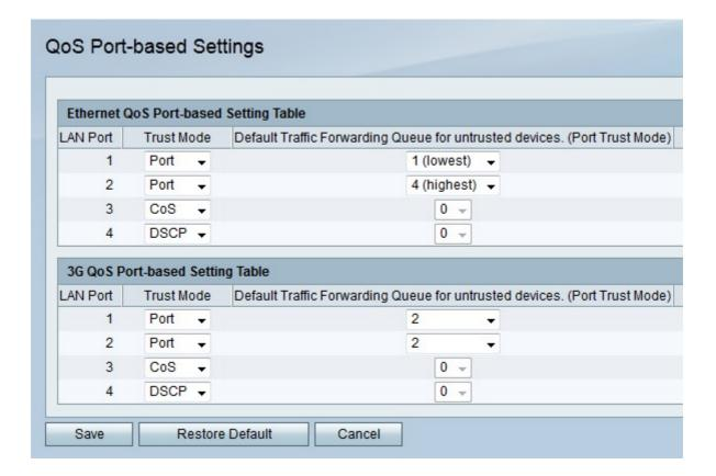
Step 2. From the Trust Mode drop-down list choose a trust mode for each LAN port. The trust mode determines how network traffic will be sent to queues.
