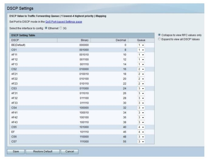
Step 2. Click the radio button that corresponds to the desired interface that you want to configure DSCP values for in the Select the Interface to Config field. This option is based on the interface that supplies internet to the RV215W.
