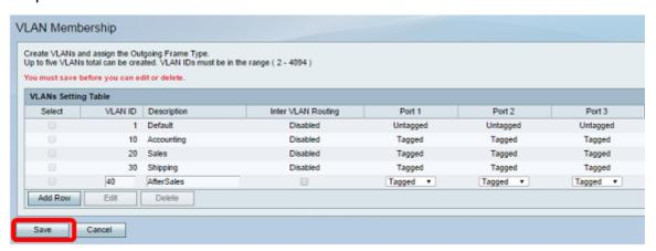
You should now have successfully added a VLAN to your RV Series Router. A confiirmation massage that configuration settings have been saved successfully will appear at the top portion of the VLAN Membership page.
