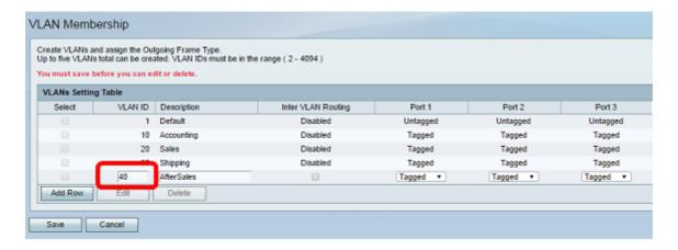
Step 4. Enter a description for the VLAN in the *Description* field. In this example, AfterSales is entered.
