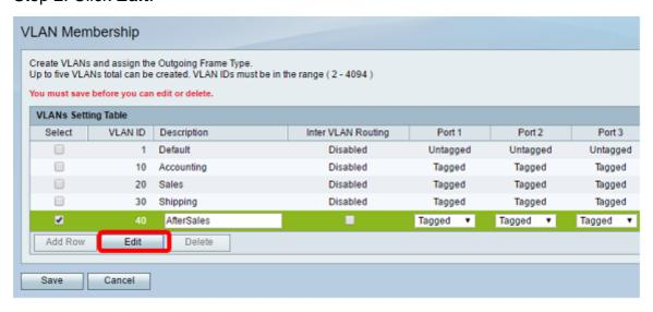
Step 3. (Optional) Check the check box to disable inter-VLAN routing. If inter-VLAN is enabled, you will need to assign an IP address to the VLANs that will be included in the routing capability.
