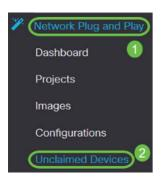
Step 2. Locate the device under *Unclaimed* devices and select it.
