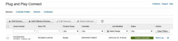
Step 16. To see if the device has checked in to the FindIT Manager, go to FindIT Manager. Navigate to **Network Plug and Play > Unclaimed Devices**.
