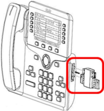
Step 5. Connect the other end of the spine connector to the second KEM.
