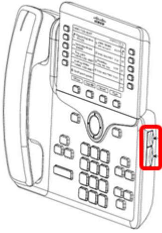
Step 4. Connect one end of the spine connector to the first KEM.
