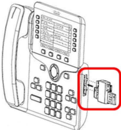
Step 5. Connect the other end of the spine connector to the KEM.
