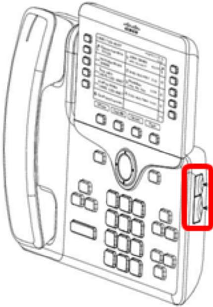
Step 4. Connect one end of the spine connector to the phone.
