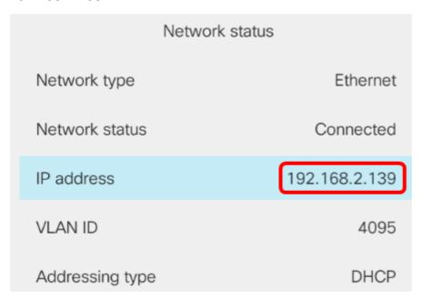
Step 5. On your computer, launch a browser and enter the following format in the Address bar: http://<phone\_ip>/admin/upgrade?<schema>://<serv\_ip[:port]>/filename then press the **Enter** key.
