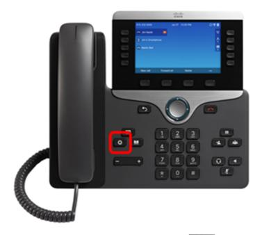
Step 2. Using the Navigation cluster button, navigate to **Status** and press the **Select** softkey.
