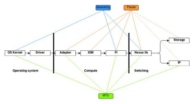
This diagram is meant as a breakdown of components a frame passed through on the way via the FlexPod environment. It does not reflect complexity of any of the blocks and is simply a way to memorize where particular features should be configured and verified.
