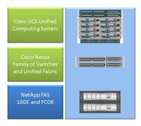
The most common FlexPod consists of a Cisco UCS B-series chassis connected via Fabric Interconnects (FIs) to Nexus 5500 switches to NetApp filers. Another solution, called the FlexPod Express, uses a UCS C-series chassis connected to Nexus 3000 switches. This document discusses the most common FlexPod.
